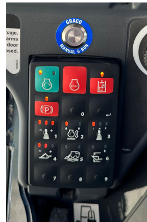
Optional Remote Run button identifies if the lubricator is cycling or if there is a warning or an error
