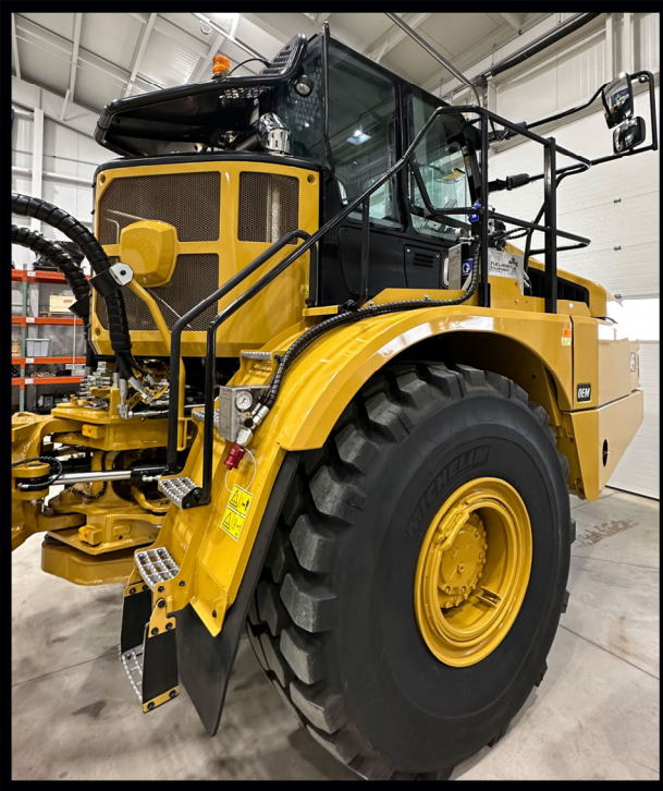
RH Side Auto-Lubrication System
