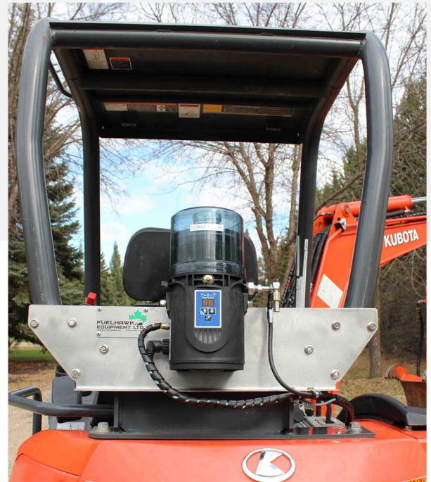
Bolt on bracket designed as to not compromise ROPS/FOPS certifications
